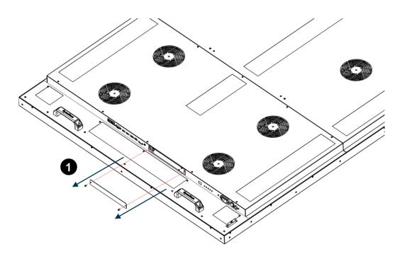
2. Insert the SDM module into the display and fasten screws. Make sure the SDM properly installed to avoid causing the devise destruction.
